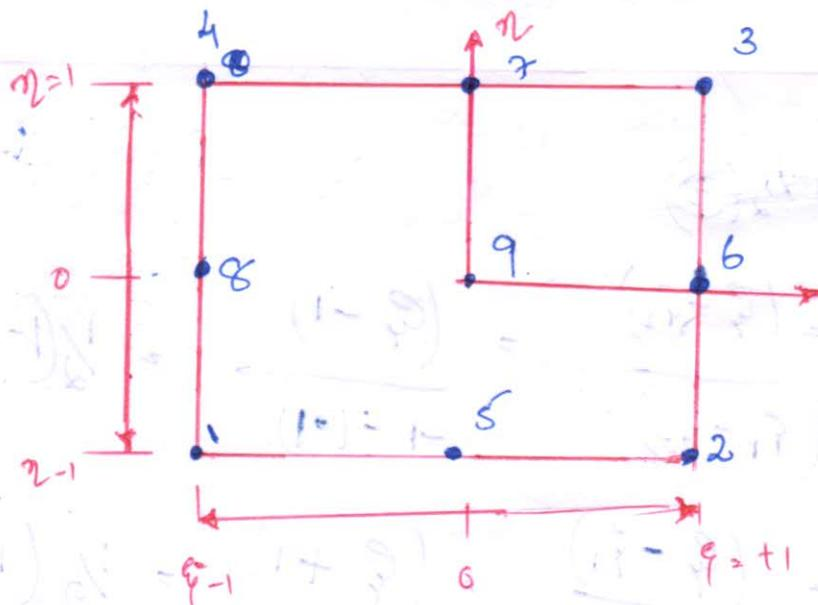
In the similar way, to the derivatives of four node rectangular element, we can derive the shape function for the nine node rect. elem.
